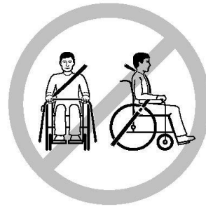
Incorrect seat belt position
