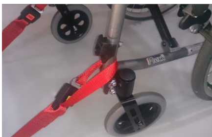
Fitting the Front Restraint
