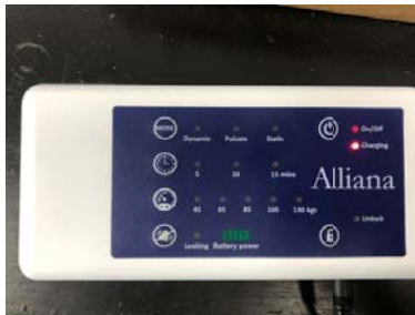
Pump are charging but power is off
