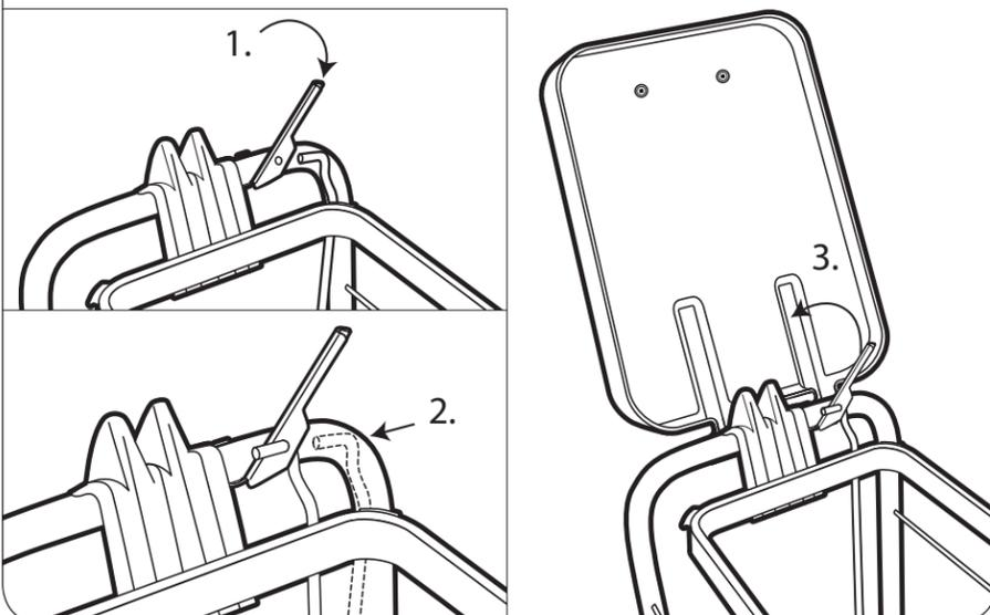
5. 1. Use a marker to indicate where you should drill. Move the lid lift lever away for easier access. A 5/32" (4 mm) bit is required on your drill. After drilling, push the lid lift lever back to the plastic lid.
