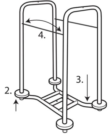
2. 1. Turn structure upside down. Ensure that cart side frames are fully inserted, but do not go past cart base frame.
