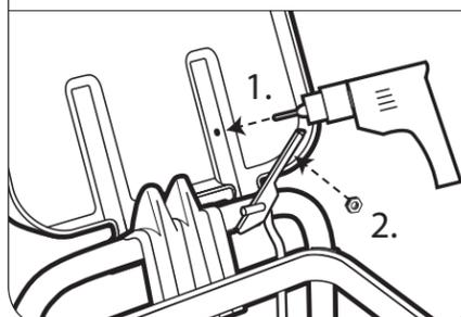
6. 1. Position the foot pedal retaining clip into recessed space. Attach with two screws. Only tighten enough to ensure that screws are fully inserted in plastic. Overtightening might strip plastic.
